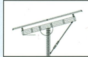
Seasonal tilting structure with turn buckle with struts
